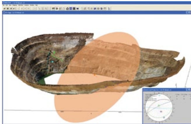
A Sirovision generated 3D mosaic of an open pit showing digitally mapped structures.. Photo courtesy of CAE Mining.
