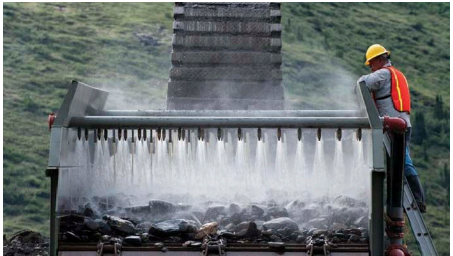
DEROCKER, washed oversize rock exiting articulating deck 2. Photo courtesy of RMS-Ross.
